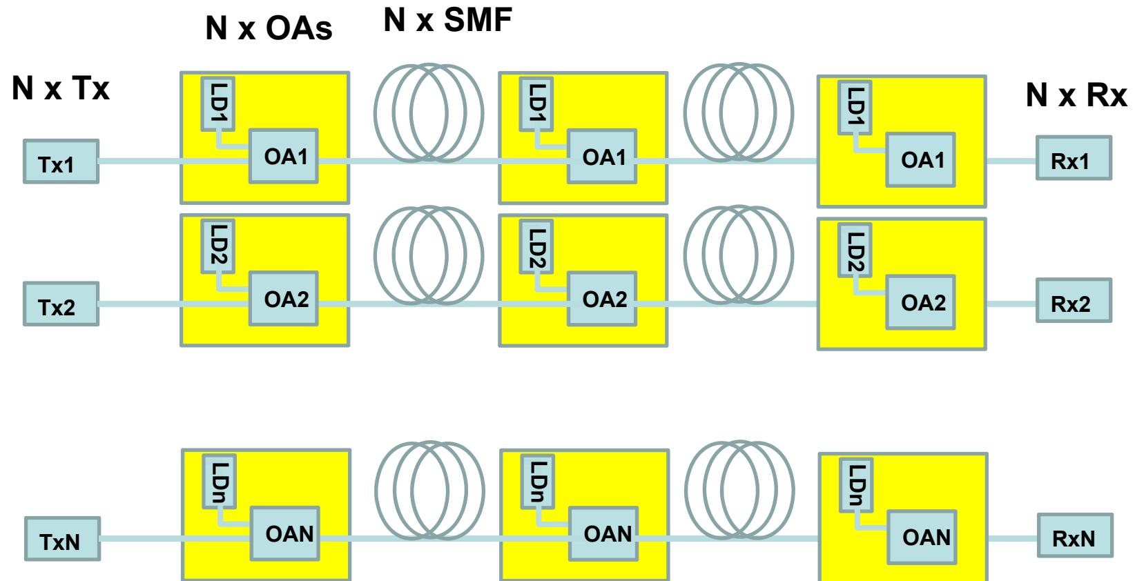
Once optimised transmitters/receivers adopted further capacity scaling can only be achieved by lighting new fibers at an effectively fixed cost per bit
