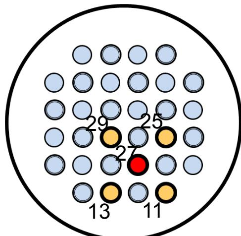
Example signal allocation for core #27 measurement
