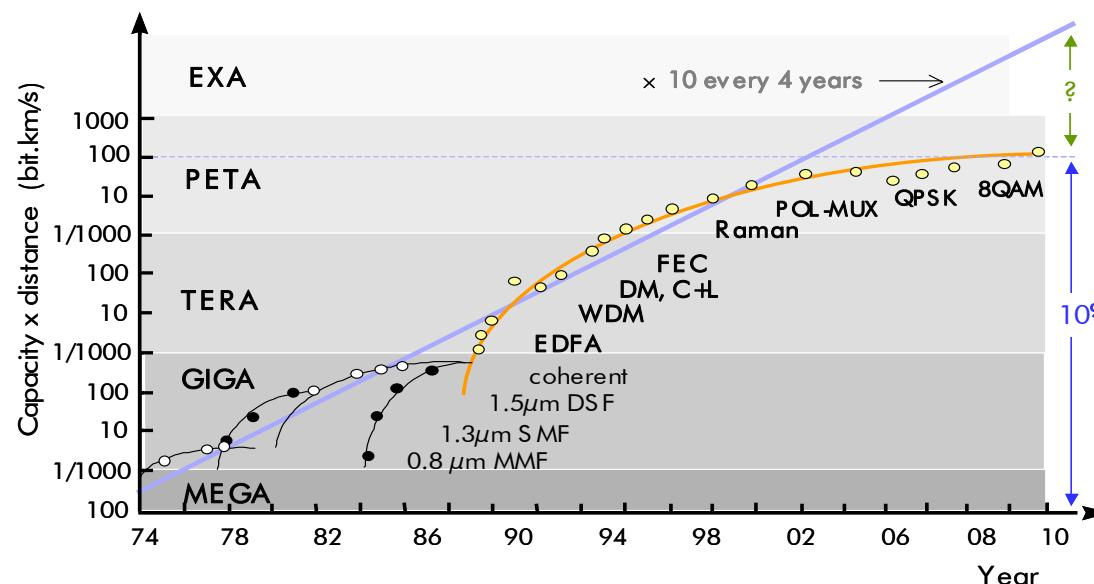
Saturation in single-mode fibre transmission capacity looming
